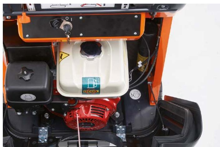
A large opening bonnet gives good access to the main areas for daily maintenance: fuel tank, air filter, engine oil level, battery, and battery isolator switch (when present) are easily reachable.
