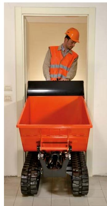
With a minimum overall width of only 758 mm (for all versions) the KC70-4 efficiently transports material through gates and doorways, between houses, buildings and many other narrow spaces. This makes it the perfect mini-dumper for renovations and urban areas.
