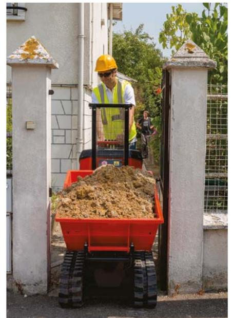
Like the other models of the product family, the Kubota KC70HD/VHD-4 has been designed to work in confined area. The variable undercarriage version allows it to be driven through narrow spaces when minimum width is set (758mm overall width) and insure excellent stability when the undercarriage is extended to the maximum position (1058mm).
