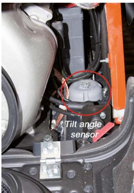
A warning buzzer turns on when the skip is at a certain level if the slope angle is more than 8°. A sensor located in the engine compartment, detects the angle of the frame. A micro-switch located on the lifting arm detects the position of the skip.
