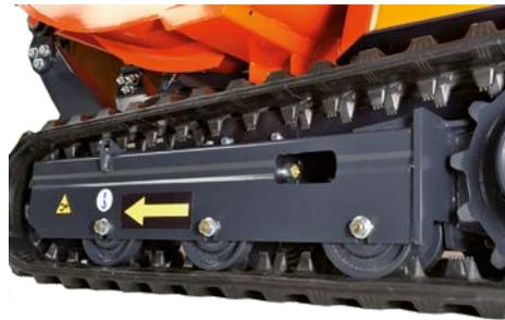
The rubber crawler is tensioned by a grease cylinder. This feature allows cushioning when foreign materials are going into the crawler. In addition, the short pitch track offers smooth drive for higher comfort for the operator.
