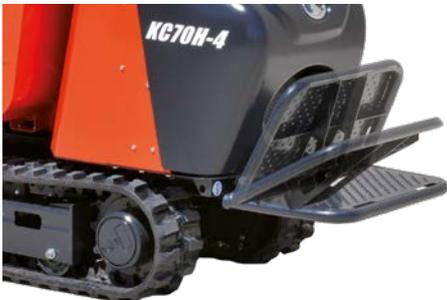
The KC70-4 features a foldable foot plate. When the plate is down, the operator can safely stand on it to operate the machine. When the plate is folded up, the overall length is reduced by 214 mm in order to gain space for transport or storage. The standing operation position makes it easier when getting on and off the machine.
