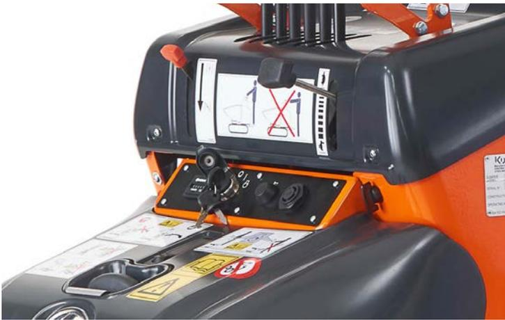
All diesel versions as well as the HD and VHD petrol engine versions, have electric starting. All other petrol versions have a heavy-duty recoil starter, which must be operated from the driving position, in combination with the automatic mechanical de-compression system ensure you easy manual starting in all conditions.
