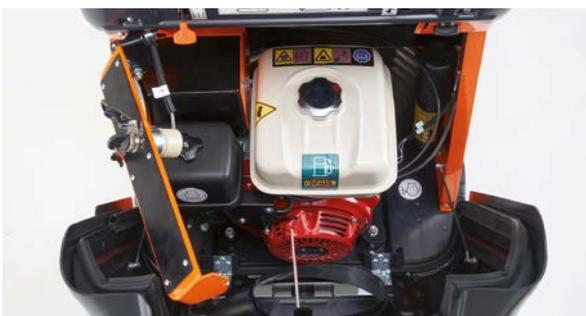
The console of petrol version can be opened for easily refueling of tank. In the diesel version, the operation is equally easy to accomplish.
