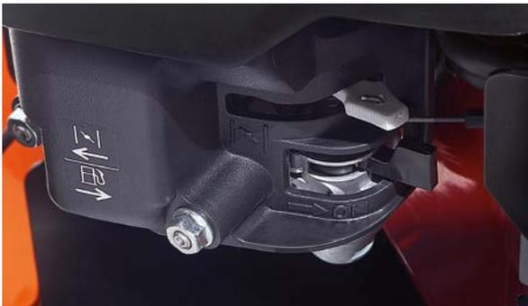
The fuel tank is fitted with a tap. If needed, the starter choke can be operated manually (petrol version).
