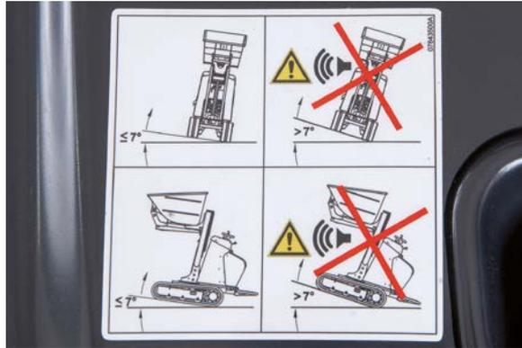
If the machine is in a slope (on the two axes) above 8°, and the skip is raised, an alarm warns of a hazard situation.
