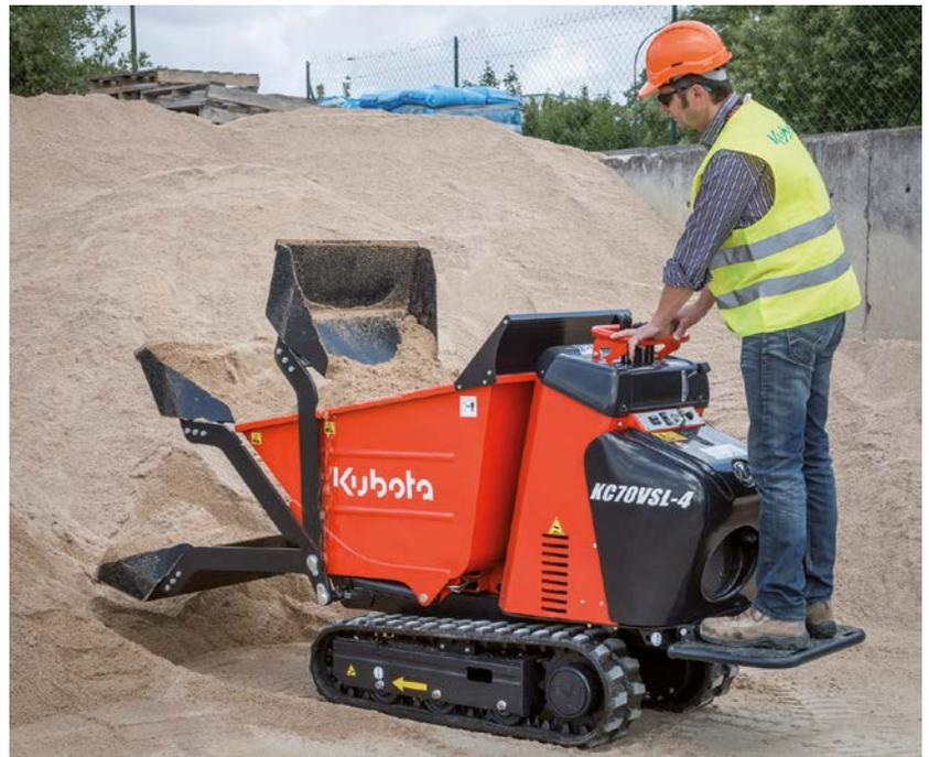
The models KC70SL-4 and KC70VSL-4 are crawler dumpers featuring a self-loading shovel. This device is very useful when you need to remove loose material (such as sand or gravel) or to clear demolition rubble. The minimum width of 758 mm allows easy access inside buildings. On the VSL version, the variable undercarriage insures good stability regardless of ground condition. The loading capacity of 700 kg makes the KC70-4 SL/VSL the ideal work mate for moving material on the job site.
