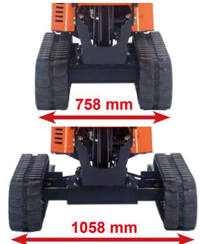
The variable undercarriage extends the overall width from 758 mm to 1058 mm. At minimum width, the KC70-4 can easily go through a standard door. At maximum width, the KC70-4 offers great stability in all conditions.
