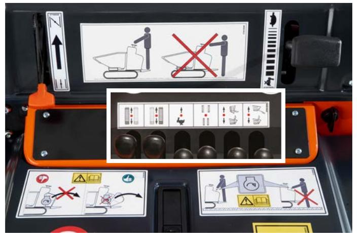
Easily visible from the operator driving position. The safety stickers give quick and easy understanding of the machines operations. This increases security and productivity. Even an occasional operator immediately understands how to use the machine.
