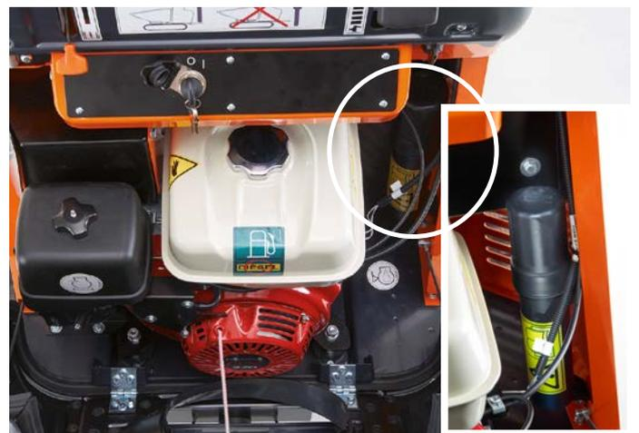
Waterproof document holder for user manuals protected in the locked engine compartment. This allows the operator to have the machine's documents always available.
