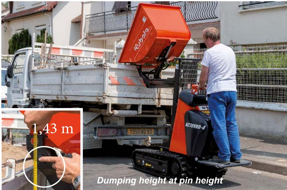
Thanks to its high dump function, the KC70HD/VHD-4 can empty its load up to 1,43m high (pin height). In addition, the dumping reach of 447mm allows easy discharge of the load from the skip, whilst leaving good clearance to the truck edge.
