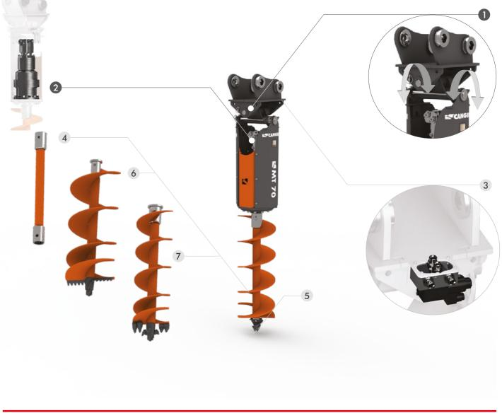
The bidirectional hydraulic auger is equipped with a transmission with epicyclical gearbox and double tilting joint. A steel envelope protects the gearbox against shocks.
